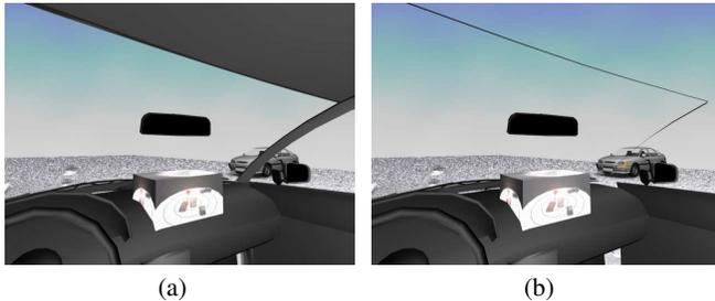
**Fig. 2.** Simulated Transparent Car Pillar Scenario (a) Original look out scene with A pillar (b) Look out scene with transparent A pillar
