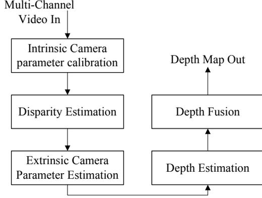
Fig. 4. The Flow Chart of the Proposed Trinocular Depth Estimation
