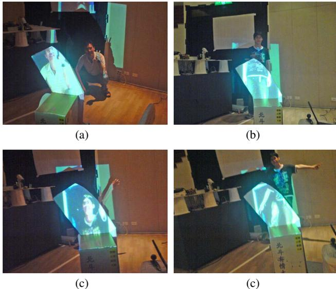
**Fig. 7.** Real-Time experimental results which make a big white pillar transparent (a)(b) A man hiding behind the pillar (c)(d) A man standing behind the pillar
