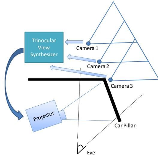
**Fig. 3.** The function diagram of the transparent car pillar
