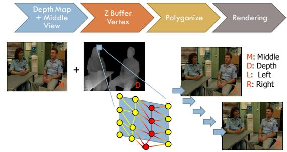
Fig. 6. Texture mapping Free Viewpoint Depth Image Based Rendering Algorithm
