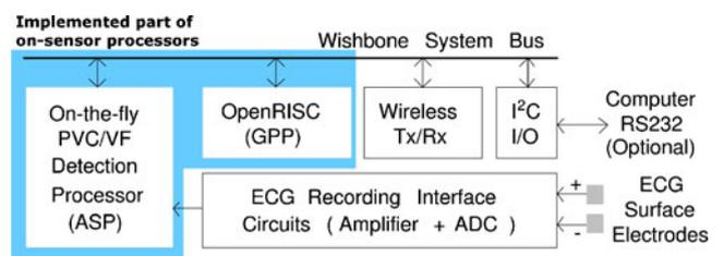
**Figure 4** The architecture of the proposed system with the on-chip ASP and GPP.
