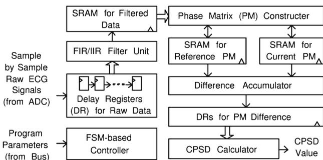
**Figure 5** The block diagram of the integrated ASP for CPSD acceleration.
