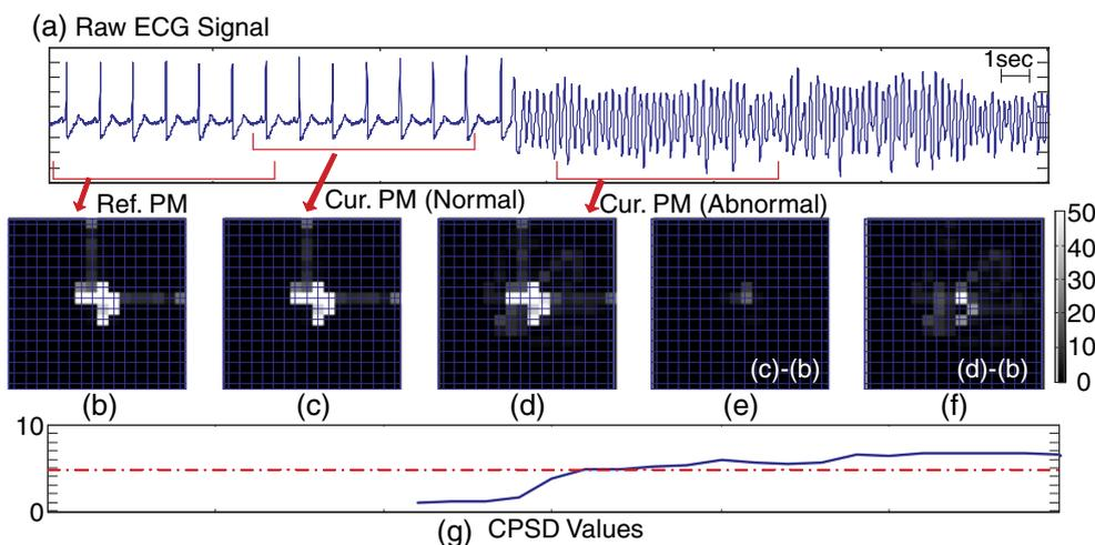
**Figure 1** The illustration of CPSD algorithm. **a** is the ECG signal derived from normal into VF. **b** is the phase space matrix constructed from normal ECG signal in the training state and served as a reference in the testing stage. **c** is the phase space matrix constructed from normal ECG signal in testing, while **d**
