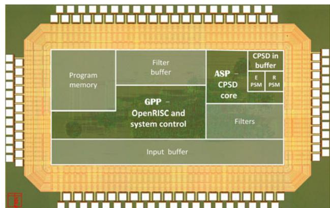
**Figure 7** 90 nm digital part chip photo.
