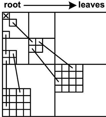
Fig. 3. Illustration of hierarchical tree in SPIHT algorithm.
