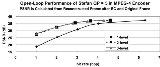
Fig. 11. Typical example of coding efficiency between different decomposition levels of DWT.
