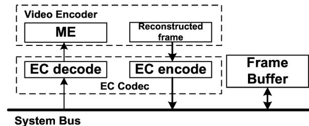
Fig. 1. Scheme for a video encoder with EC engine to reduce external access when ME and MC.
