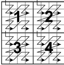
Fig. 14. Sequence of encoding/decoding one coding pass in one bit-plane. The number indicating the clock cycle corresponding region is processed, and the arrows indicating the sequence of coding within one clock cycle.
