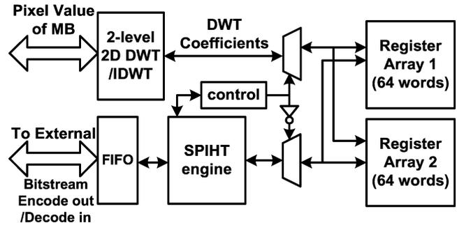
Fig. 13. Alternative system architecture avoiding bubble cycles.
