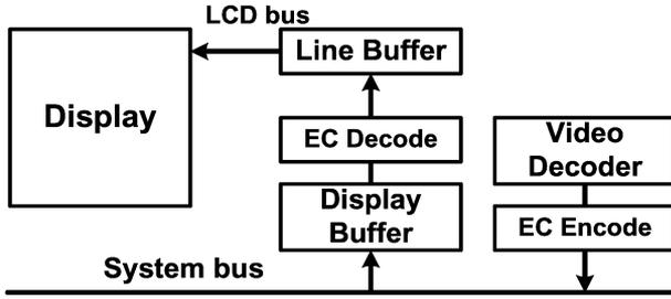
Fig. 2. Scheme for decoding system with EC engine to reduce the system bus and display buffer access when displaying.
