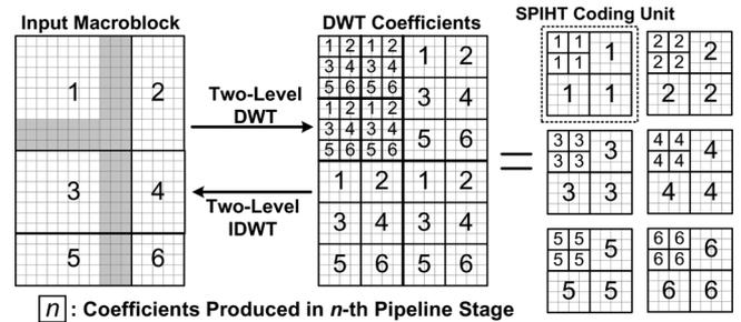
Fig. 9. Proposed four-tree pipelining scheme with encode scheduling.
