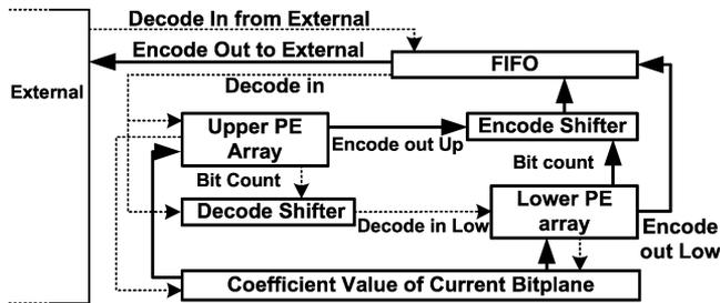
Fig. 15. Architecture of SPIHT codec engine. Solid lines indicate the dataflow of encoding, and the dashed lines are decoding dataflow.
