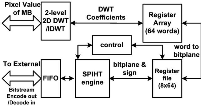
Fig. 12. Proposed system architecture for multimode EC codec engine.
