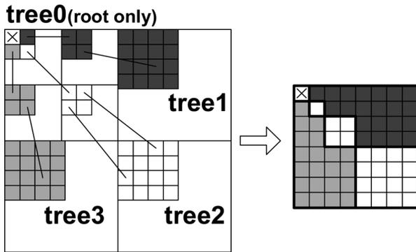
Fig. 6. Proposed algorithm takes four adjacent hierarchical trees (three complete trees and one tree without descendent) in DWT transformed coefficients as a coding unit of SPIHT engine.
