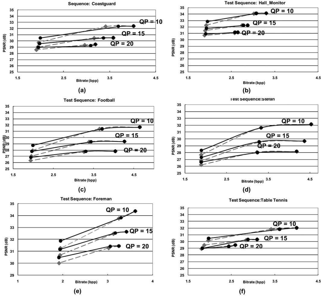
Fig. 7. Comparisons of coding efficiency of SPIHT algorithm (black solid line) and the four-tree pipelined SPIHT (gray dashed line). The test sequences comprise CIF 30 fps reconstructed videos generated by MPEG-4 simple profile encoder with different QPs. The results in the figure are the averaged coding efficiency after those sequences are processed by embedded compression macroblock-by-macroblock.
