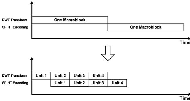
Fig. 5. Illustration of the change of encoding flow by dividing one macroblock into four coding units.
