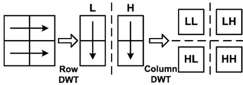
Fig. 8. Example of dataflow in single level 2-D DWT of four pixels.
