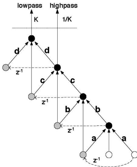
Fig. 3. SFG for lifting-based architecture of (9,7) filter.
