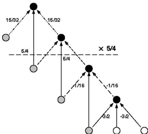
Fig. 11. Flipping structure of integer (9,7) filter.
