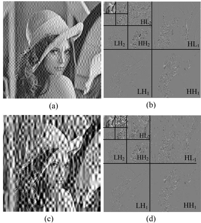
**Fig.1 Single bit-error on different subbands with bit rate=1.0.**
