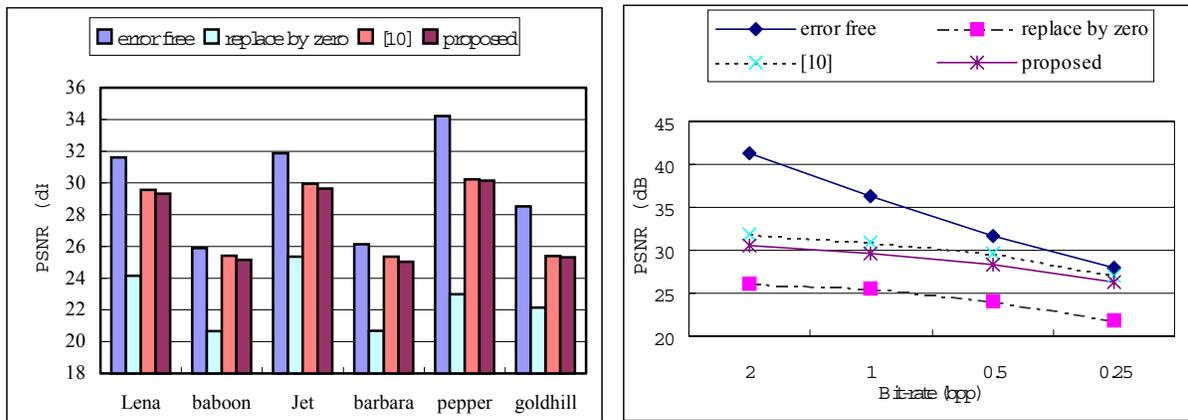
Fig.6 (a) The result of the test images with BER=10e-3 and bit rate=0.5bpp in HL<sub>2</sub> subband, and (b) objective comparison of "Lena" image with various bit rates HL<sub>2</sub> subband
