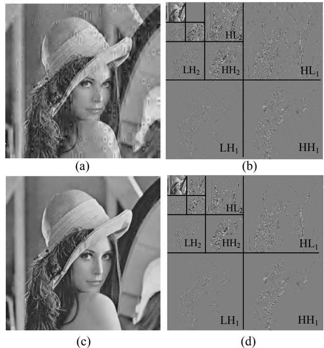
**Fig.2 (a)(b) Reconstructed image by zero replacement. (c)(d) The original image.**
