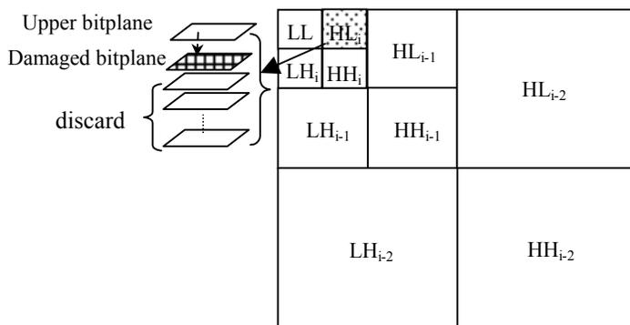
(b) The structure of DWT coefficients.
