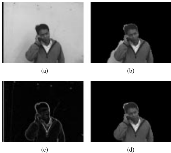
Fig. 6. Effect of gradient filter. (a) Original image. (b) Segmentation result of the original image. (c) Gradient image after applying the morphological gradient operation. (d) Segmentation result of the gradient image.
